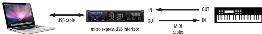
Figure 3-1: An example of connecting a single MIDI device to a MOTU micro express interface. Connect the device’s MIDI OUT and MIDI IN ports to the interface.
